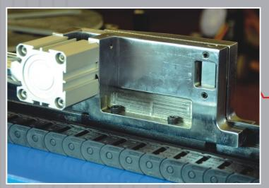
The clamp unit which holds the rule and feed in the machine provides high length accuracy. The unit is controlled with a servo motor.
