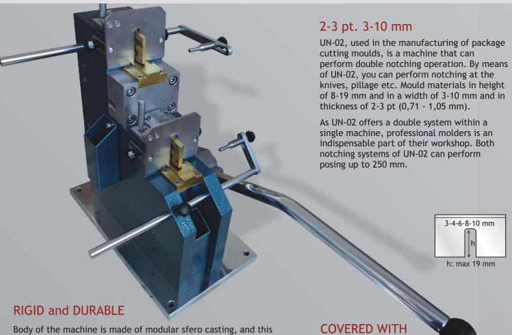
Body of the machine is made of modular sfero casting, and this added strength and durability to the machine. As the machine has a rigid body, it is able to resist the impacts that will occur during the bending operation for many years.
